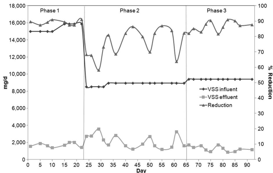
Fig. 4. VSS of the influent, effluent, and percentage reduction
