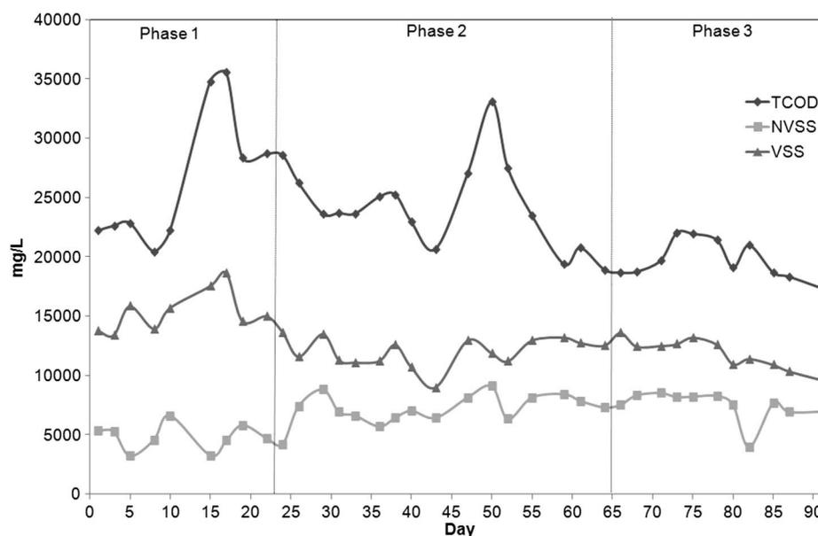
**Fig. 2.** TCOD, VSS, and NVSS levels in the reactor during the three phases
