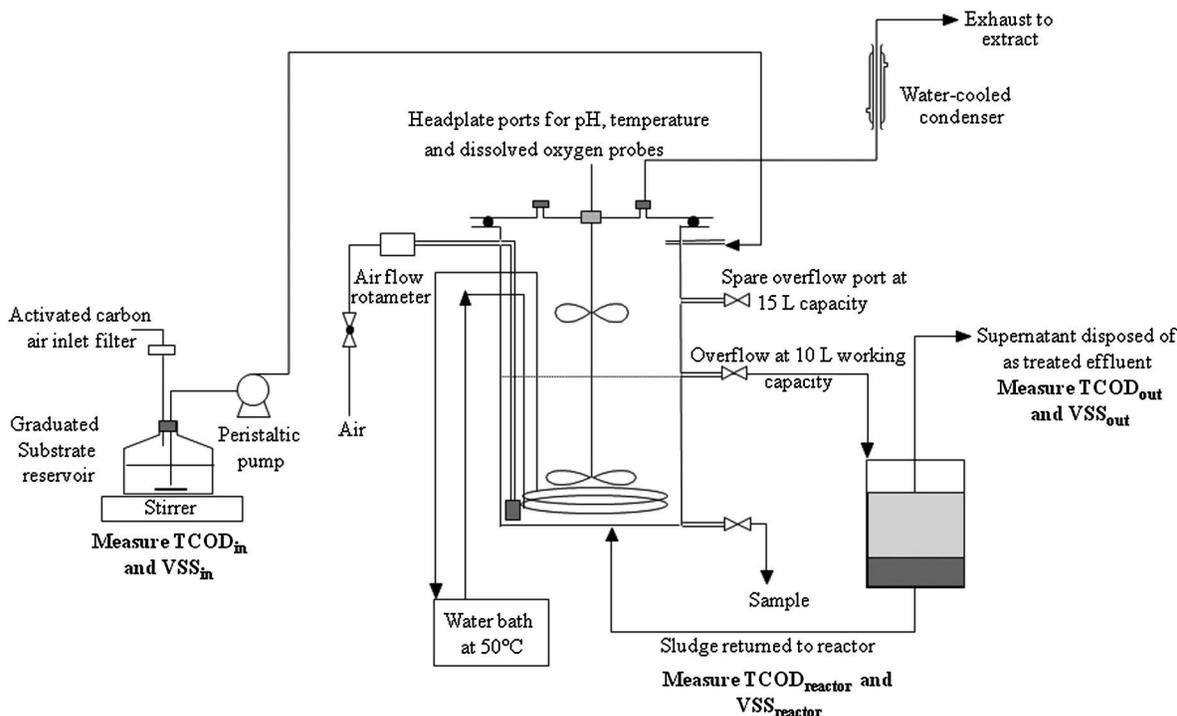
Fig. 1. Experimental setup for aerobic thermophilic experiments
